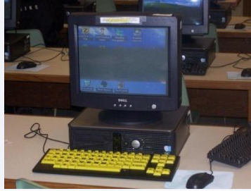
Large bright yellow keys on this keyboard allow individuals with visual or motor impairments access to computer use
